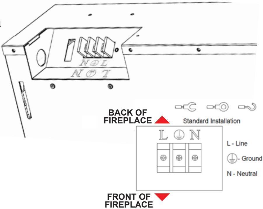
**NOTE: A dedicated 20 Amp (or higher) breaker is required.** This fireplace must be electrically connected and grounded in accordance with local codes. In the absence of local codes, use the current CSA C22.1 CANADIAN ELECTRICAL CODE in Canada or the current ANSI/NFPA 70 NATIONAL ELECTRICAL CODE in the United States.
