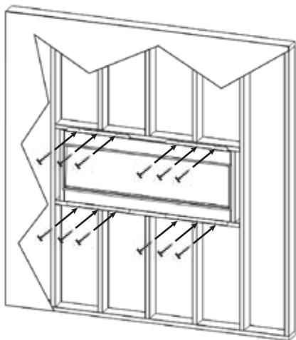
2. Install L Metal mounting brackets to the top and bottom of the fireplace with supplied screws.
