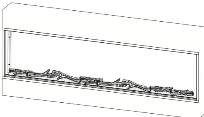
4. The front glass can now be installed, by installing bottom of glass in track, then tilt towards fireplace. After placing the front glass it can be secured with screws.
