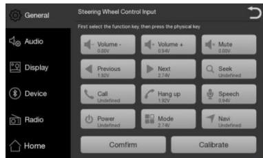
After the **【Calibrate】** is touched, select the keys you wanted to set. Pressing one steering wheel key when the screen pop a window with
