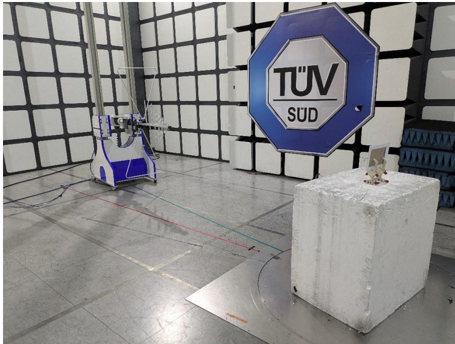
Figure 48 – Test Setup 30 MHz to 1 GHz
