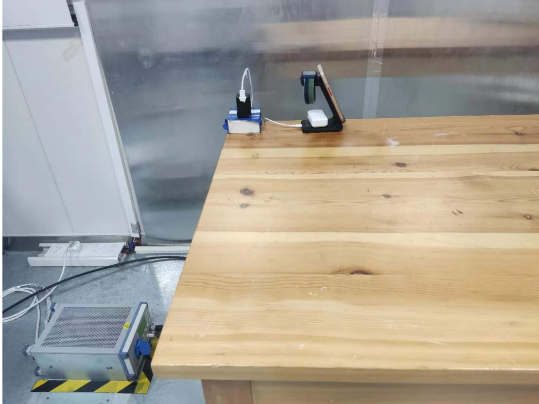
Conducted emission test setup
