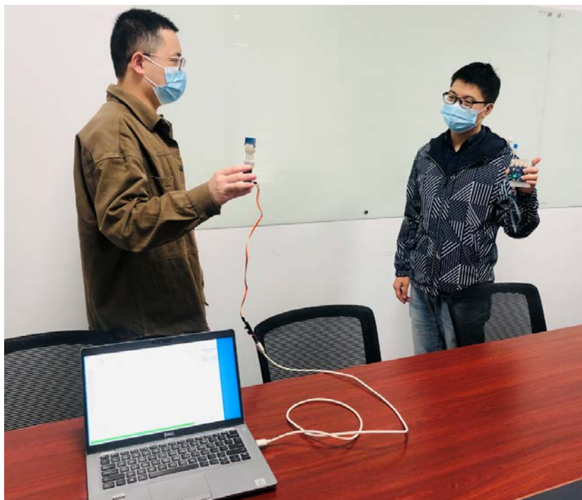
Figure 9 Example of setup of Ranging and AoA test in Standalone mode
