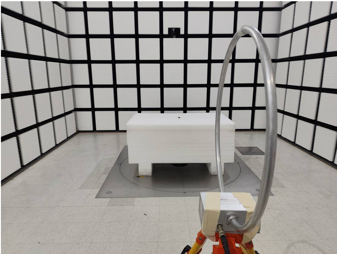
Radiated Emission Below 1GHz View Ground-parallel-left ear
