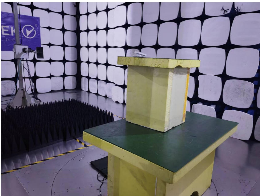
Spurious Emission Test Setup (Above 1GHz)
