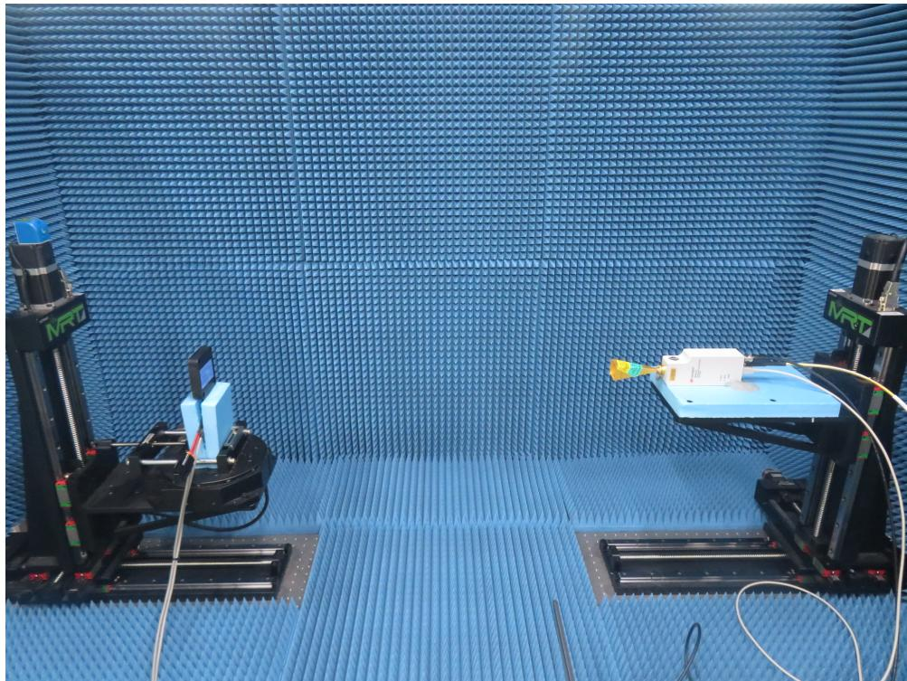
Description: Radiated Emission Test Setup for 55GHz ~ 90GHz
