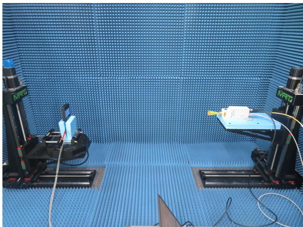
Description: Radiated Emission Test Setup for 90GHz ~ 110GHz
