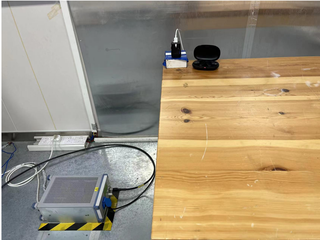
Conducted emission test setup
