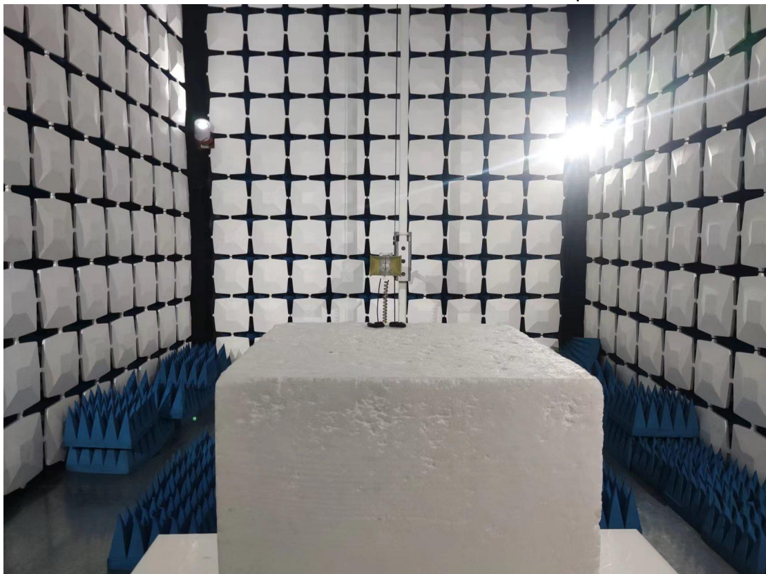
Above 1GHz for radiated emission test setup
