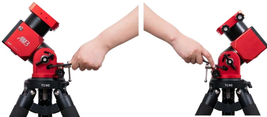
Pull the mount head, you'll notice the two hex screws are sliding to the bottom place of the inner slideway, while the latitude scale is currently pointing at 45°. Retighten the hex screws on both sides.
