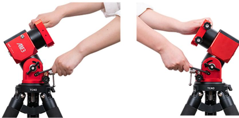
Now the mount is at Gear 2, you need to re-tighten the two hex screws to avoid looseness and any possible damage. Gear 2 gives an adjusting range of the latitude scale from 45° to 90°. Don't forget to lock the tension grip after you complete adjusting the latitude scale.
