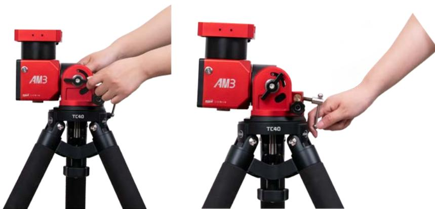
Use the hex wrench to anticlockwise rotate the two hex screws. Make sure they are totally loose before you go to next step.
