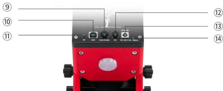
⑨ **Auto guide:** Can be used to connect a ST4 guide cable.
