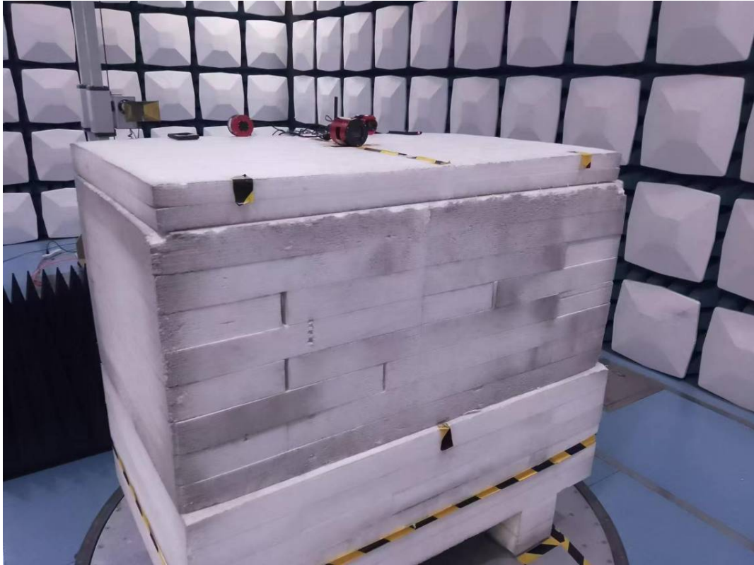
Radiated Emission 18-26.5GHz View
