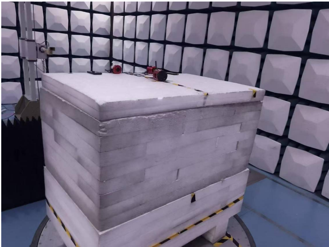
Radiated Emission 18-26.5GHz View
