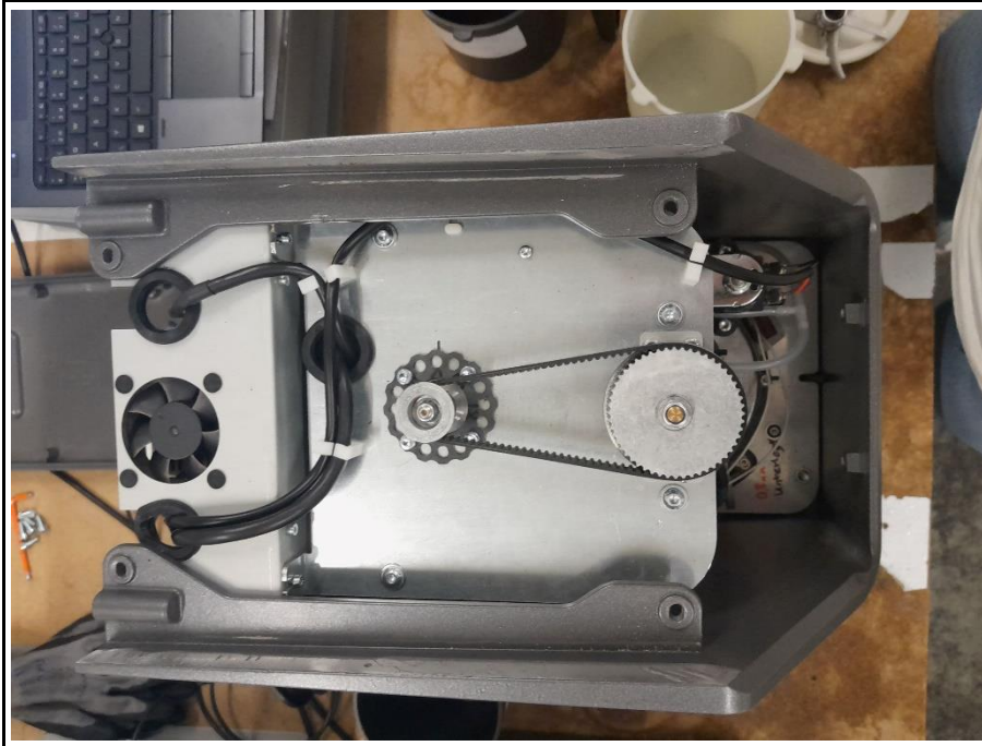
EUT WITHOUT MAIN PCB TOP SIDE
