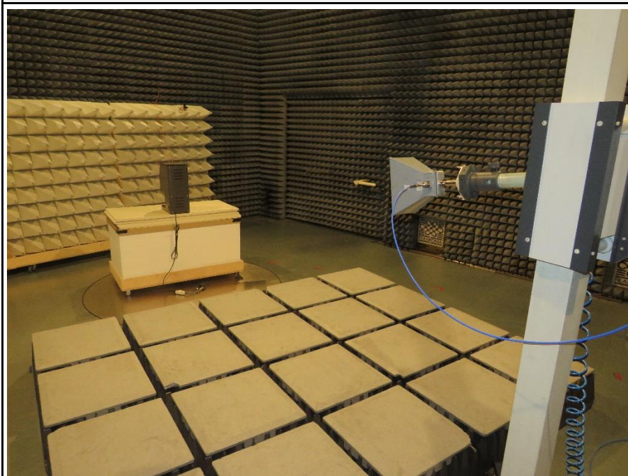
TEST SETUP – 1-15GHz
