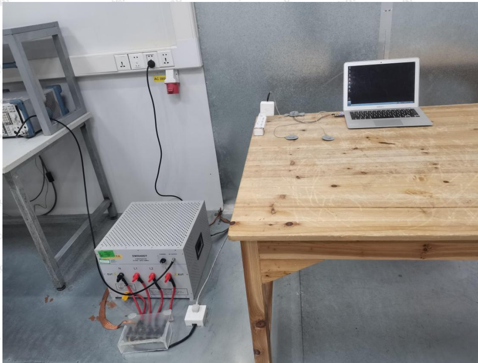
Photo of Conducted Emission Measurement
