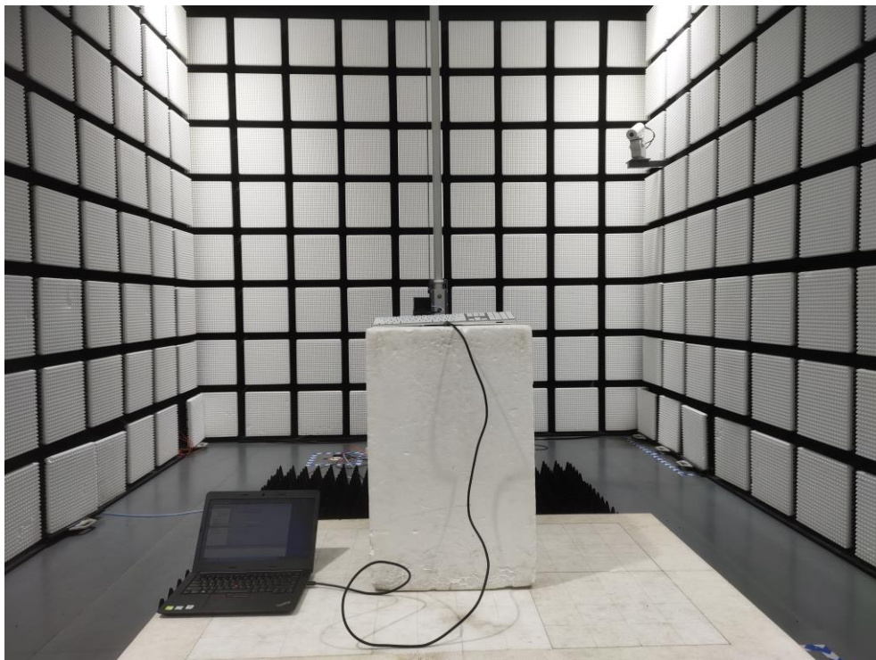
Fig. 3 Radiated emission setup photo(Above 1GHz)
