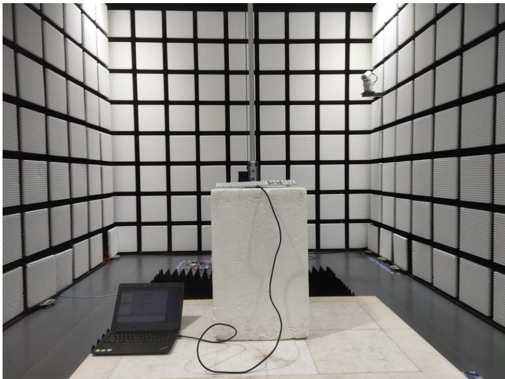
Fig. 3 Radiated emission setup photo(Above 1GHz)
