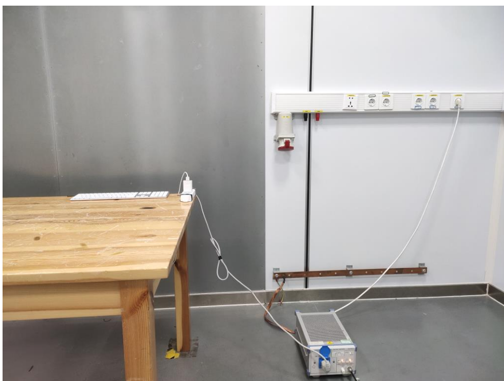
Fig. 4 Power line conducted emission setup photo
