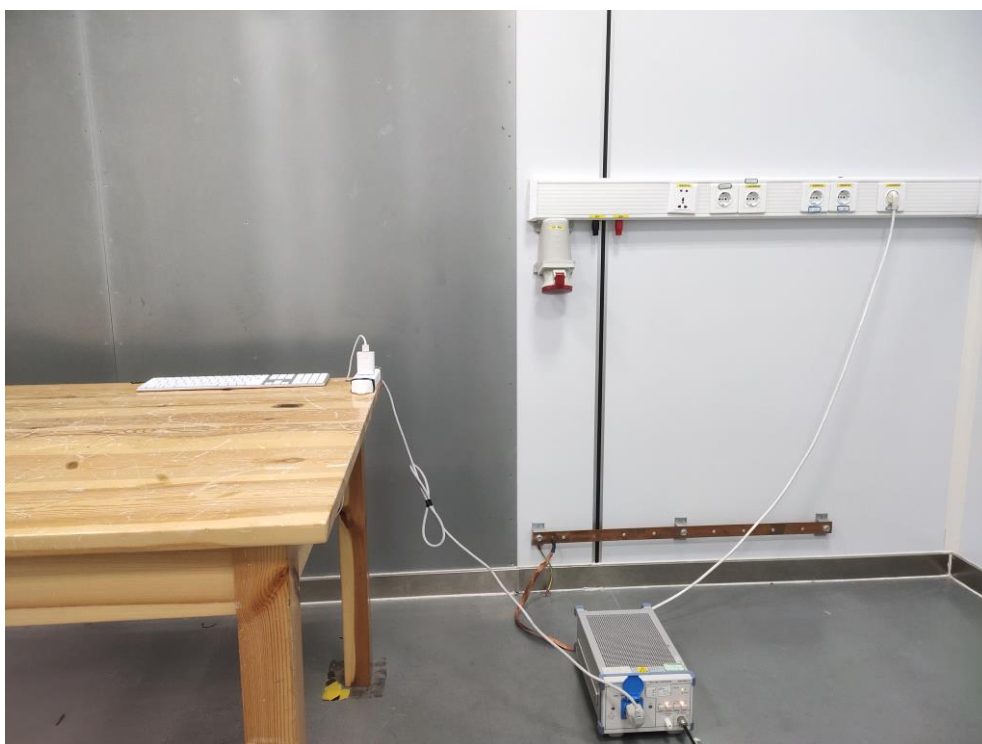
Fig. 4 Power line conducted emission setup photo
