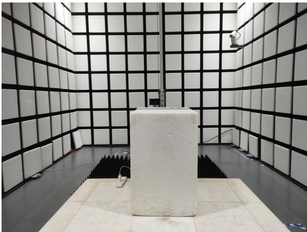
Fig. 3 Radiated emission setup photo(Above 1GHz)
