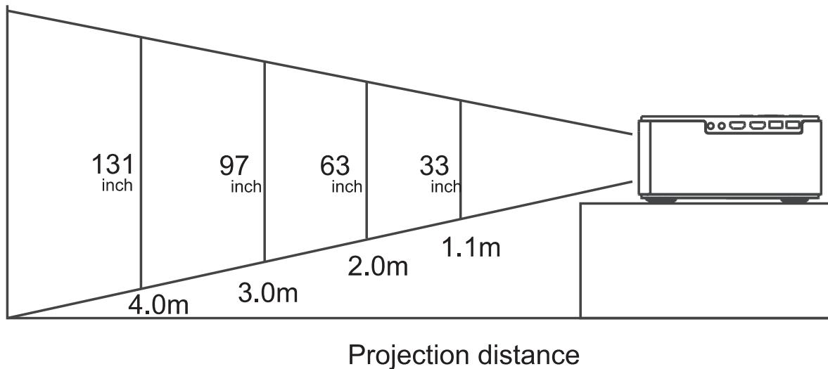
Note: The projection size and projection distance are calculated according to the projection ratio. During actual debugging, there may be deviations and please refer to the actual product.
