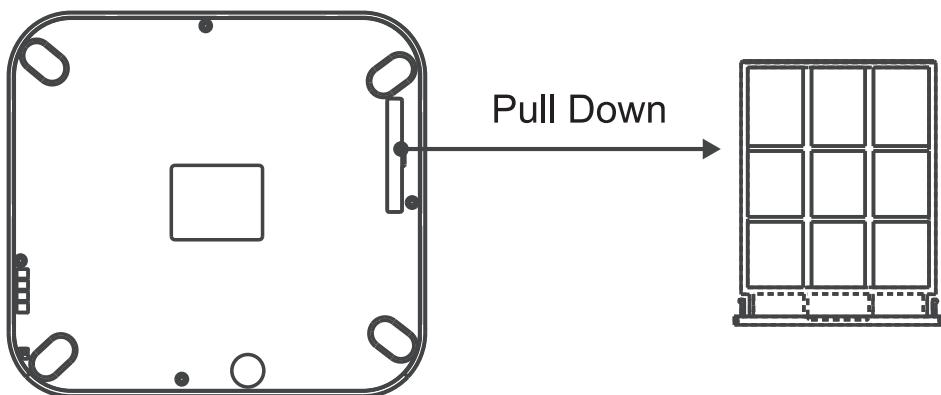
After the machine is used for a period of time, it is necessary to remove the dust-proof plate and remove the dust on it in time. Please use a soft brush to remove the dust gently. Do not wash with water ! !
