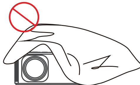
Do not block air intake vent or air outlet vent !
