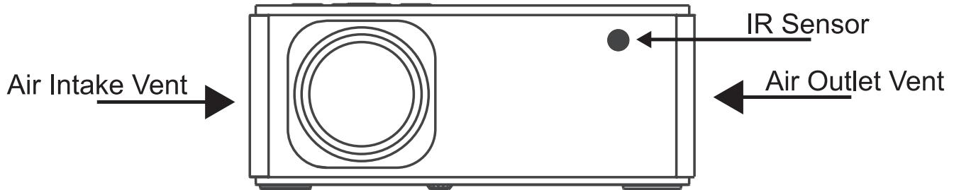
Caution: The air outlet is the cooling outlet of the machine and its temperature is higher, but it does not affect the use of the machine
