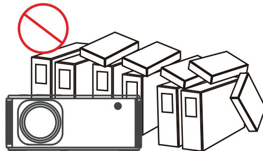
Do not install in places with poor ventilation
