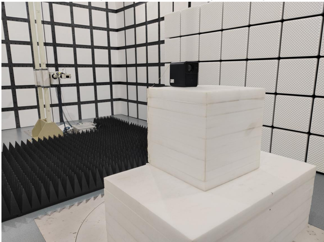
Radiated Spurious Emissions Test View (18GHz-25GHz)
