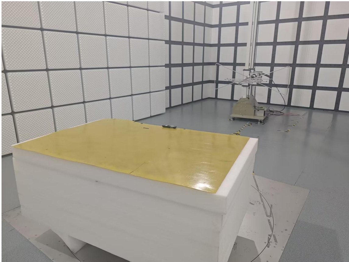
Radiated Spurious Emissions Test View (30MHz-1GHz)
