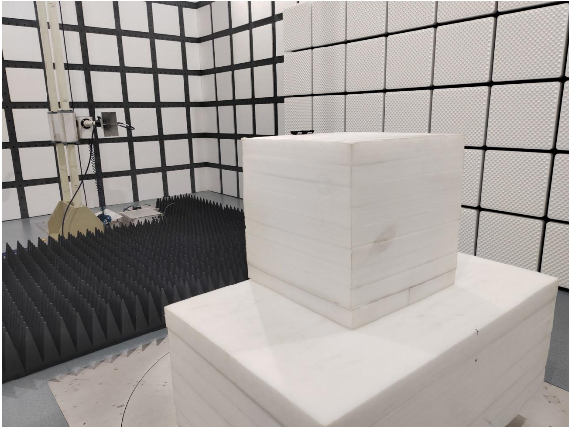
Radiated Spurious Emissions Test Front View (18GHz-25GHz)
