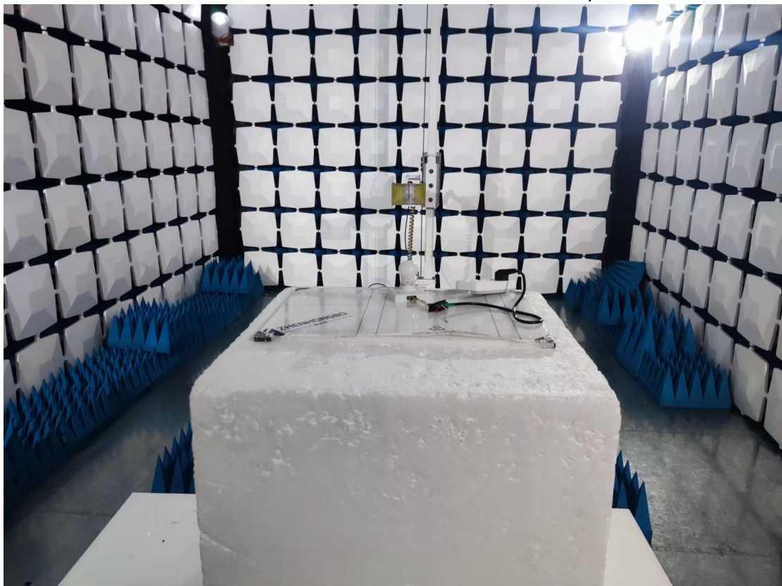
Above 1GHz for radiated emission test setup
