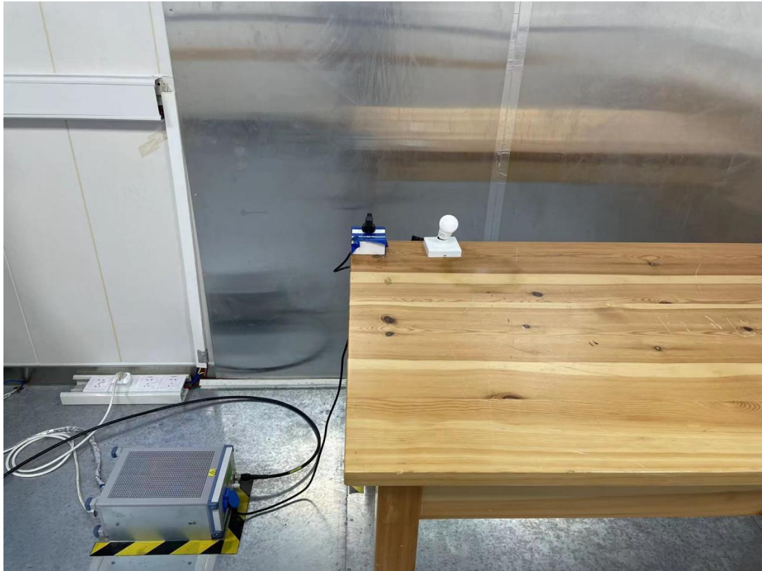
Conducted emission test setup
