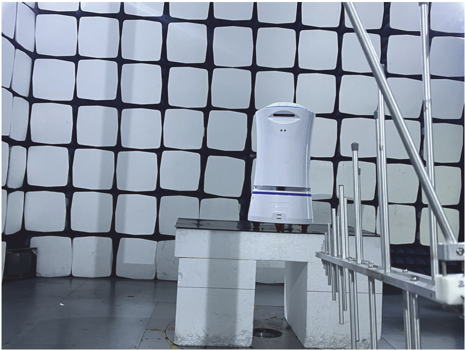
Radiation Emission Test Setup (30MHz to 1GHz)
