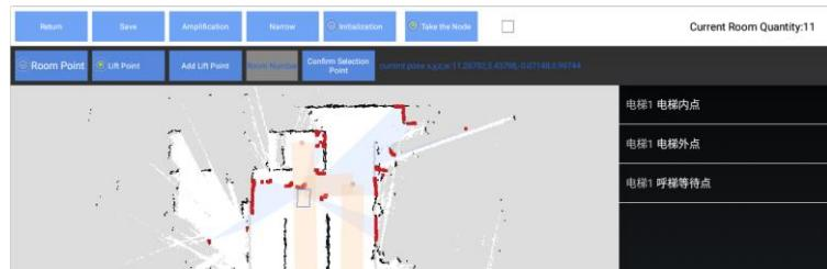
Push the machine to the corresponding elevator position, select the corresponding point name on the right, and then confirm the selected point
