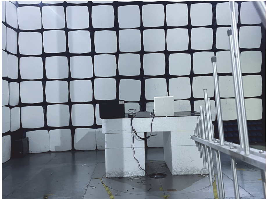
Radiation Emission Test Setup (30MHz to 1GHz)
