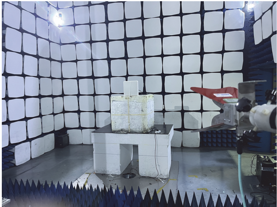
Radiation Emission Test Setup (1GHz to 18GHz)
