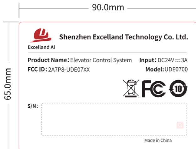
Specifications: The label shall be securely affixed to a permanently attached part of the device, in a location where it is visible or easily accessible to the user, and shall not be readily detachable. The label shall be sufficiently durable to remain fully legible and intact on the device in all normal conditions of use throughout the device's expected lifetime.
