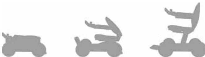
Expanding Electric wheelchair, if there is no other command, it will stop automatically after unfolding
