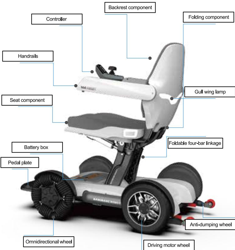
Main structural composition of products: Motor, storage battery, control system, wheel, seat, handrail and pedal
