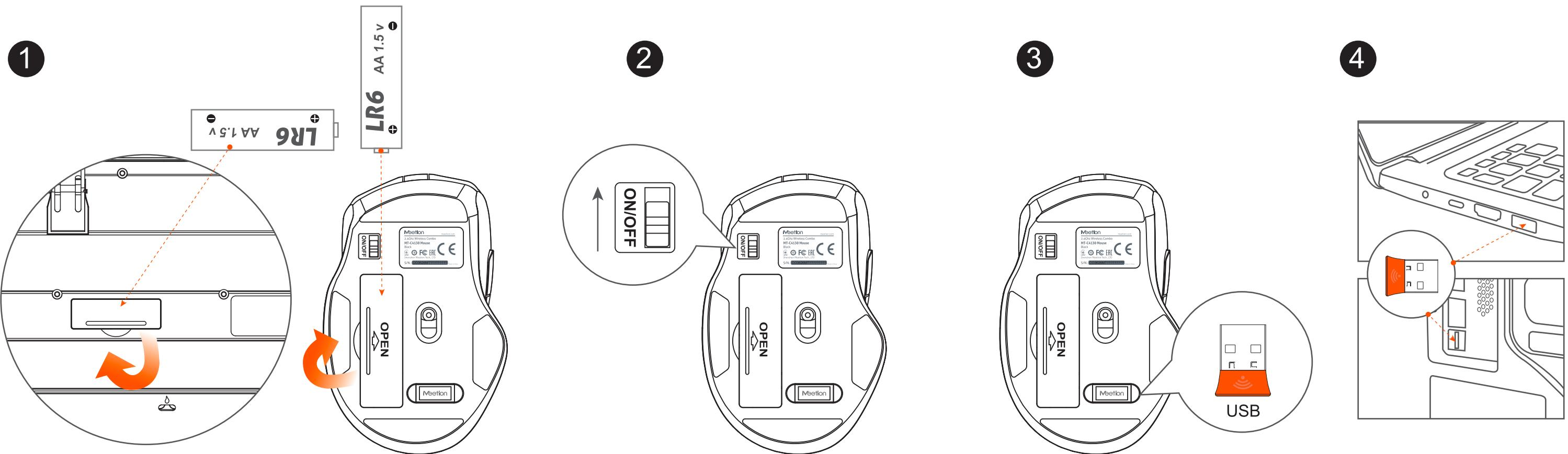
Open the battery compartment cover at the bottom of the keyboard and mouse, and insert a AA battery into each
