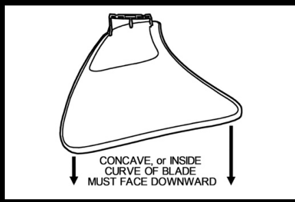
⑤ The inner curve, or concave side of fan blade must face downward (toward the ground) when installed.
