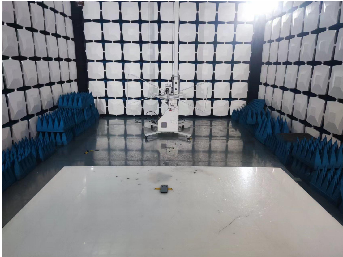
Above 1GHz for radiated emission test setup
