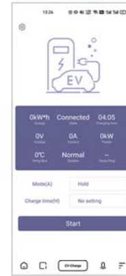
Plug in the charging gun and click the start button
