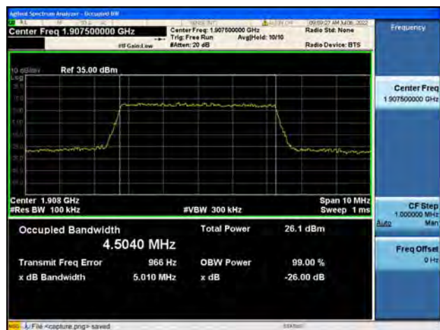
B2 / 5MHz / 16QAM/ High CH
