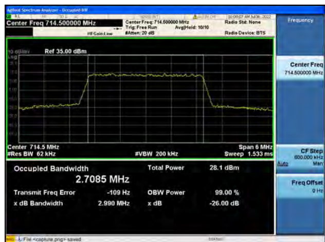
B12 / 3MHz / QPSK/ High CH
