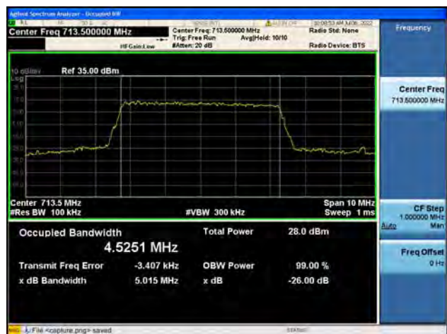
B12 / 5MHz / QPSK/ High CH
