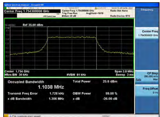
B4 / 1.4MHz / 16QAM/ High CH
