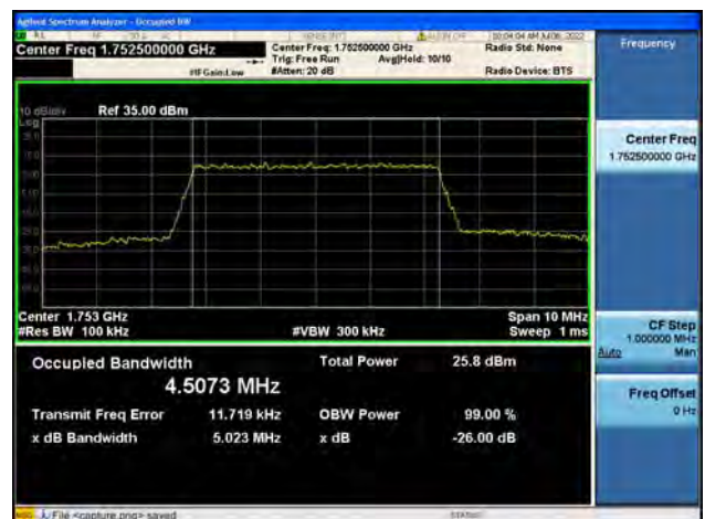
B4 / 5MHz / 16QAM/ High CH
