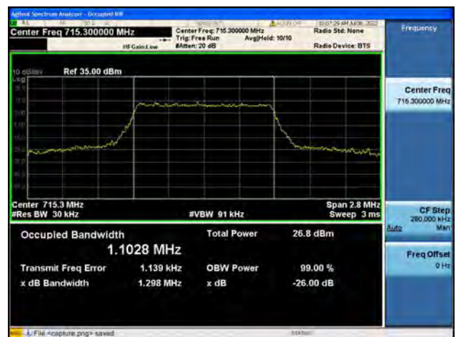
B12 / 1.4MHz / 16QAM/ High CH
