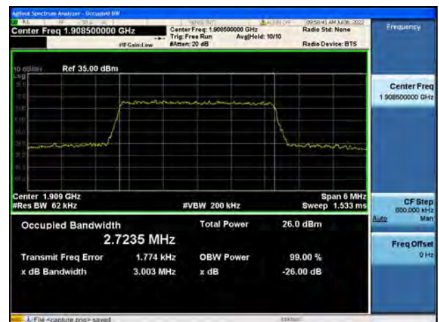
B2 / 3MHz / 16QAM/ High CH
