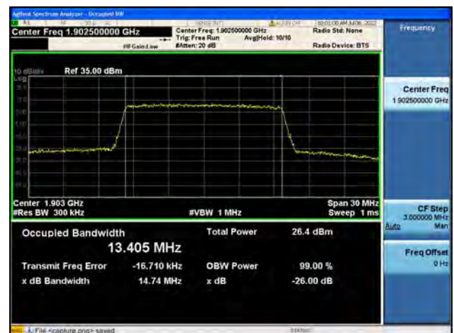
B2 / 15MHz / 16QAM/ High CH
