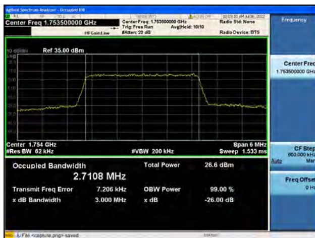
B4 / 3MHz / QPSK/ High CH
