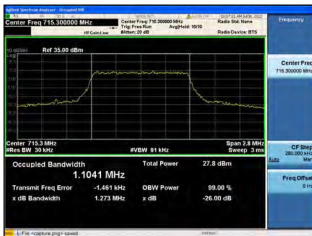
B12 / 1.4MHz / QPSK/ High CH
