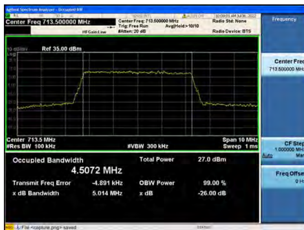
B12 / 5MHz / 16QAM/ High CH
