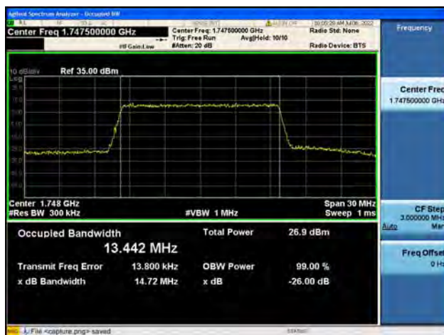
B4 / 15MHz / QPSK/ High CH
