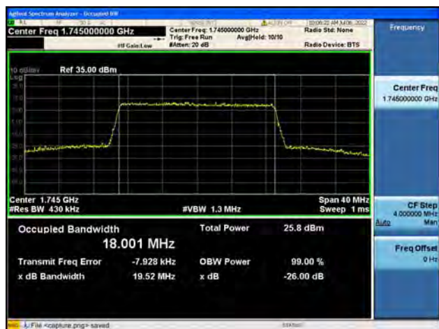
B4 / 20MHz / 16QAM/ High CH
