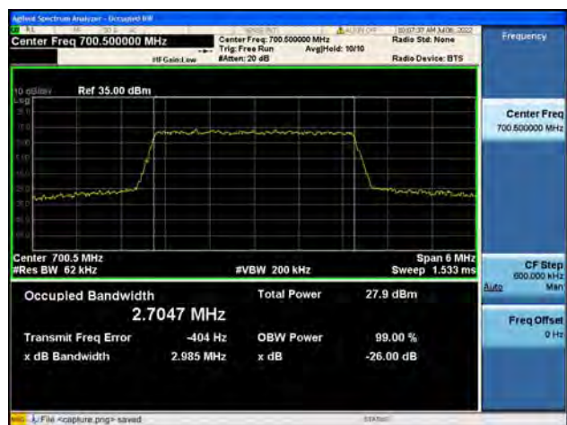
B12 / 3MHz / QPSK/ Mid CH
