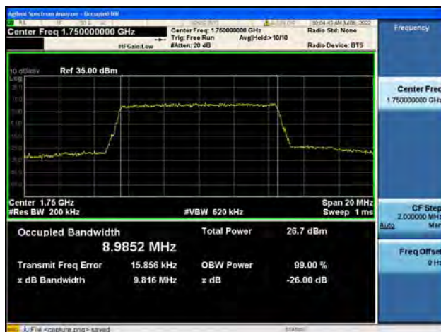
B4 / 10MHz / QPSK/ High CH
