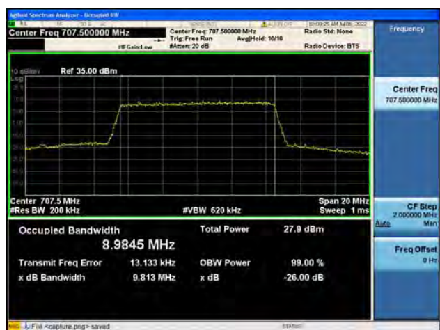
B12 / 10MHz / QPSK/ High CH
