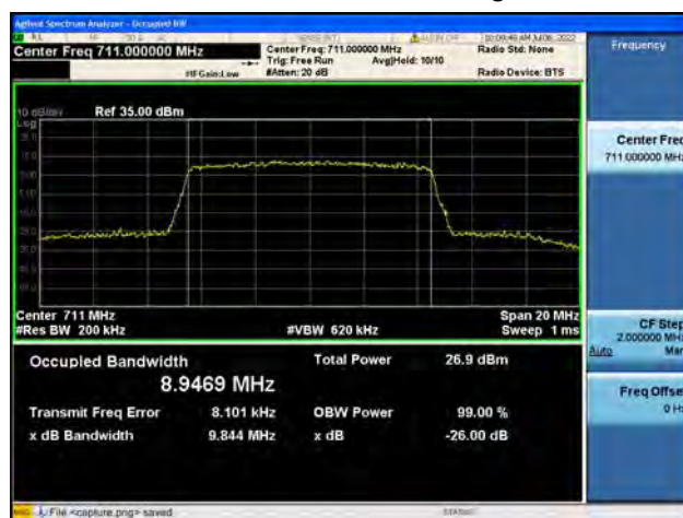
B12 / 10MHz / 16QAM/ High CH
