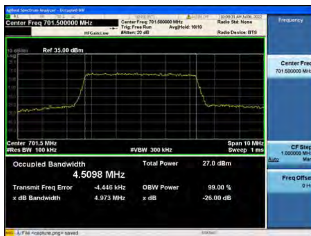
B12 / 5MHz / 16QAM/ Mid CH
