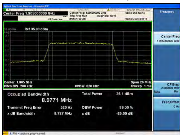
B2 / 10MHz / 16QAM/ High CH
