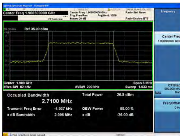
B2 / 3MHz / QPSK/ High CH
