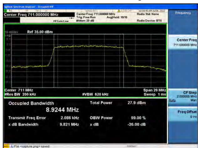
B12 / 10MHz / QPSK/ High CH
