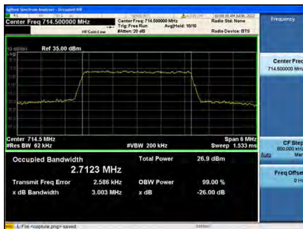
B12 / 3MHz / 16QAM/ High CH
