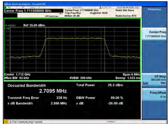
B4 / 3MHz / 16QAM/ Mid CH
