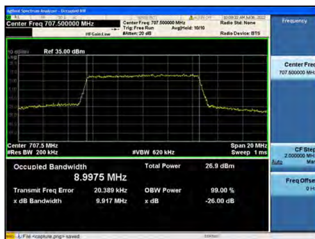
B12 / 10MHz / 16QAM/ High CH
