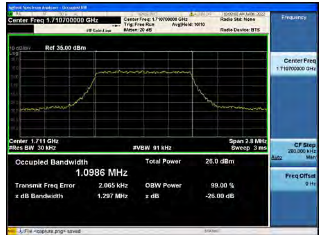
B4 / 1.4MHz / 16QAM/ Mid CH
