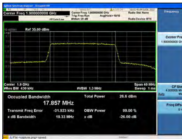
B2 / 20MHz / 16QAM/ High CH
