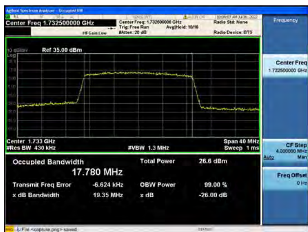
B4 / 20MHz / 16QAM/ High CH
