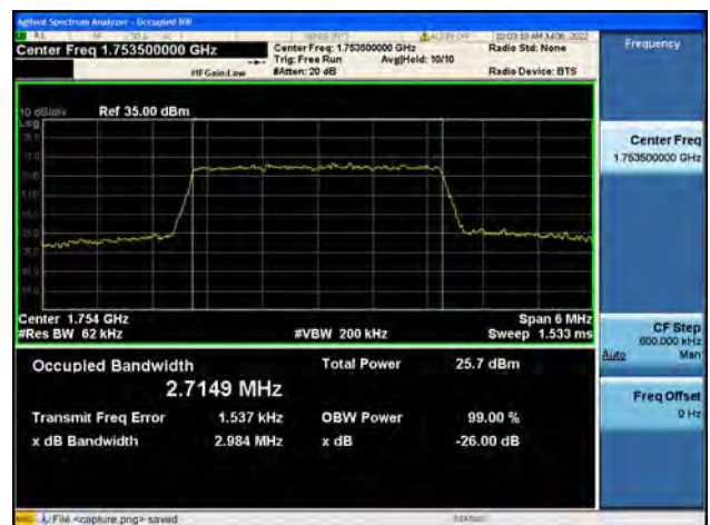
B4 / 3MHz / 16QAM/ High CH
