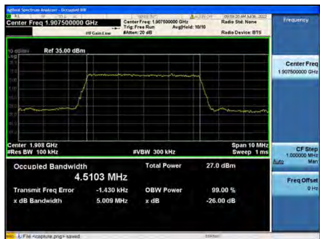
B2 / 5MHz / QPSK/ High CH
