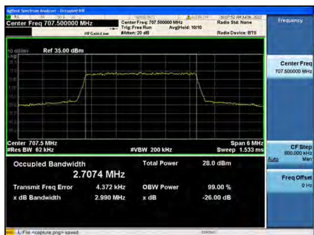
B12 / 3MHz / QPSK/ High CH
