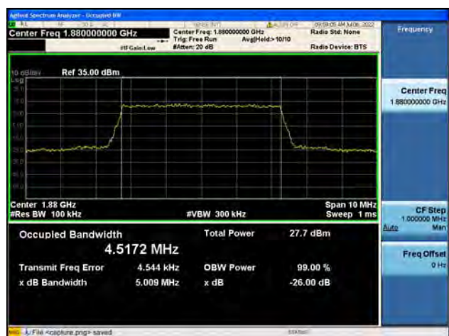
B2 / 5MHz / QPSK/ High CH
