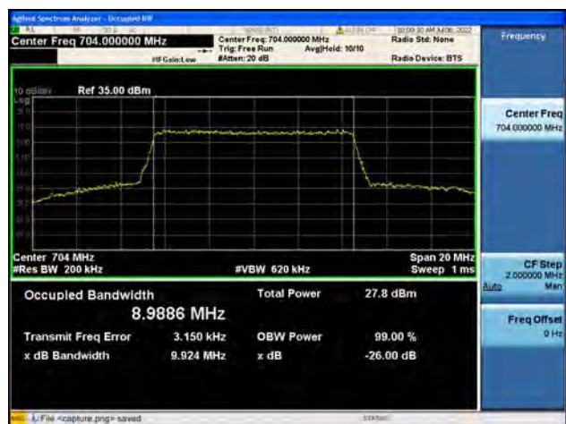
B12 / 10MHz / QPSK/ Mid CH
