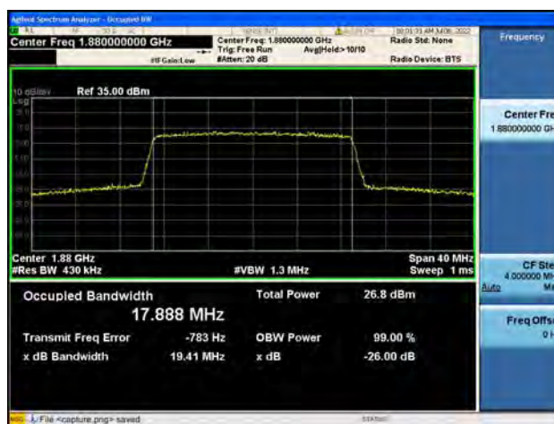
B2 / 20MHz / 16QAM/ High CH
