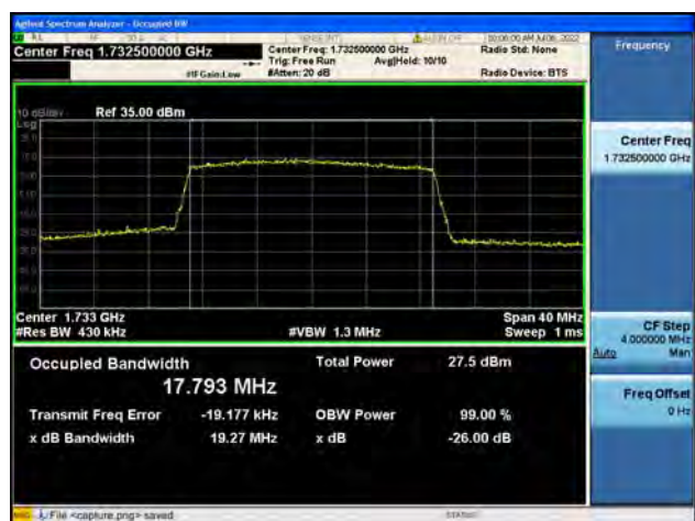
B4 / 20MHz / QPSK/ High CH
