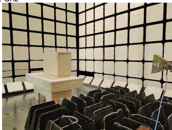
Fundamental & Spurious Emission & Restrict band radiated emission – FCC 15.231(b) and 15.205: 1 GHz – 6 GHz
