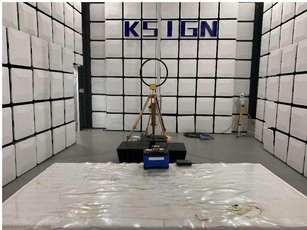
Radiated Measurement (Above 30MHz)
