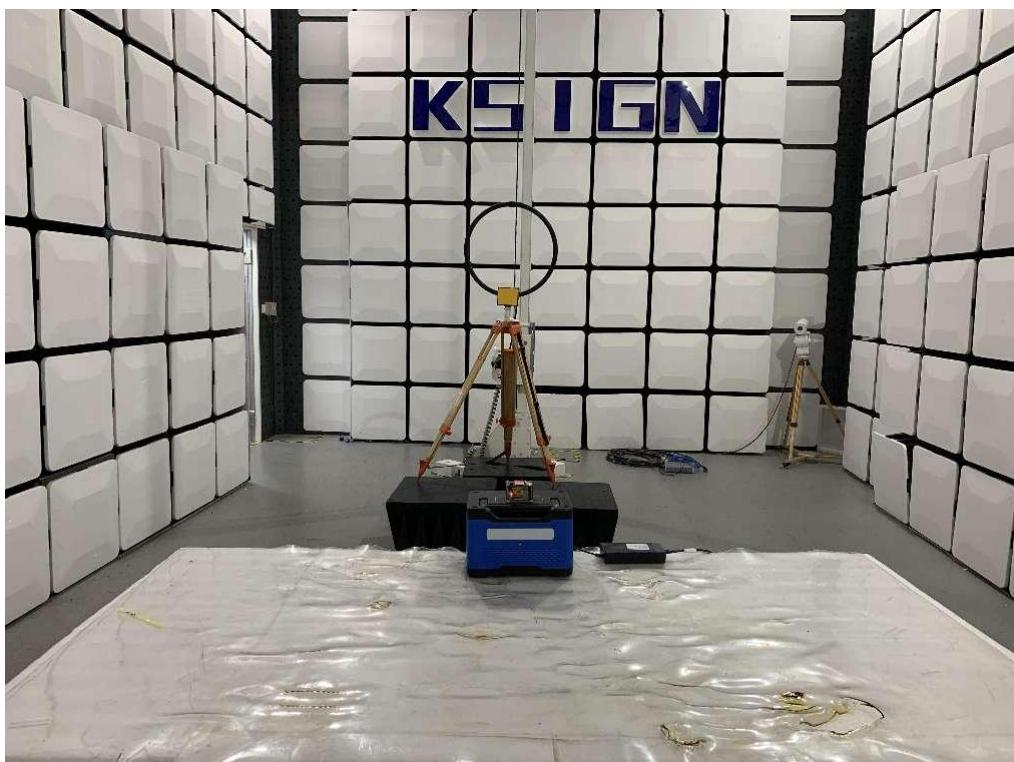
Radiated Measurement (Above 30MHz)
