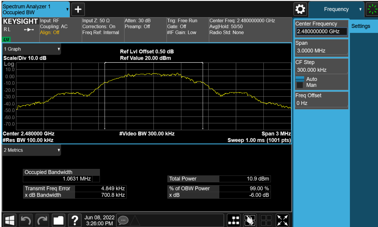
Figure 6: 6dB Bandwidth, 2480MHz
