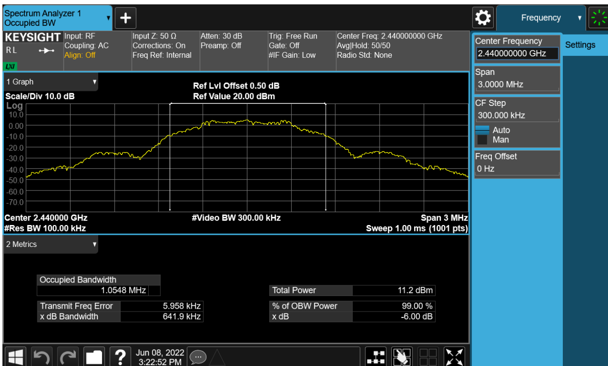
Figure 5: 6dB Bandwidth, 2440MHz
