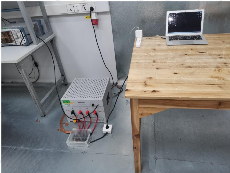
Photo of Conducted Emission Measurement
