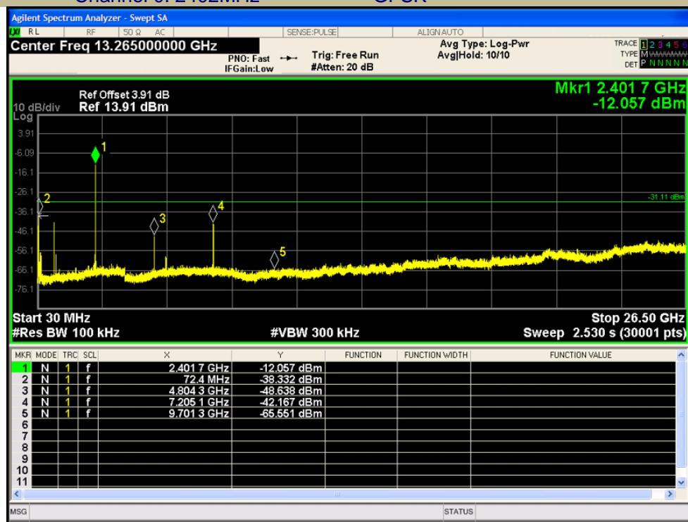
Test Model Band-edge Conducted Emissions
