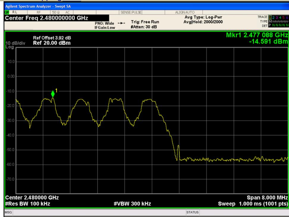
Test Model      Band-edge Conducted Emissions
