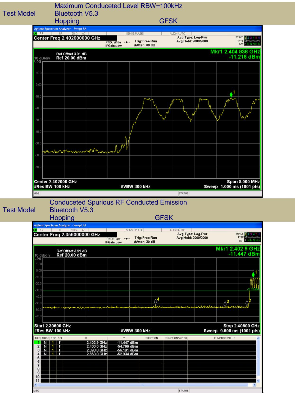
Test Model      Band-edge Conducted Emissions
