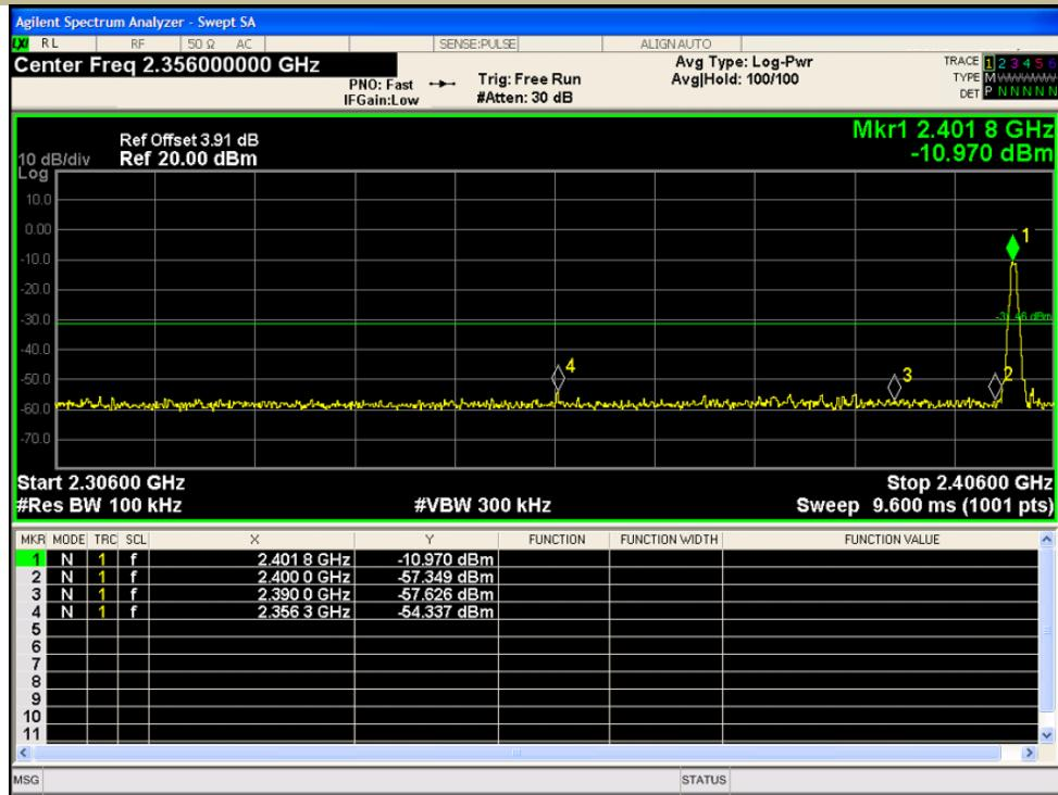
Test Model Maximum Conducted Level RBW=100kHz
