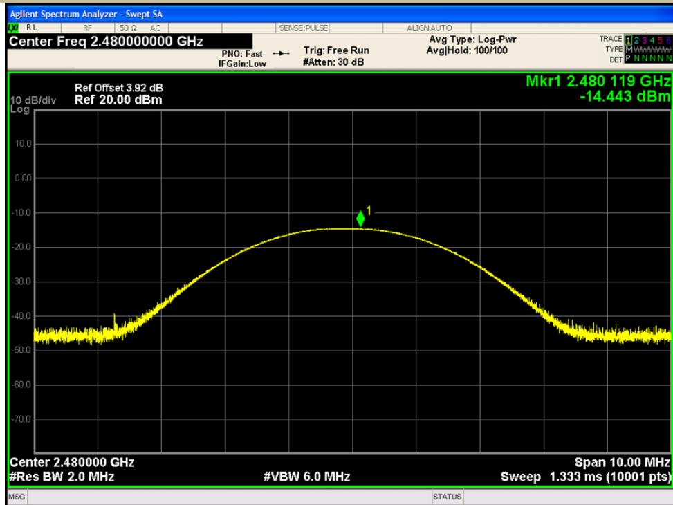
Test Model Maximum Peak Conducted Output Power
