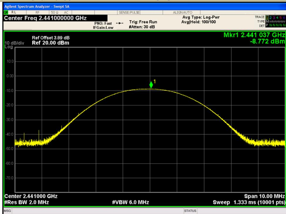
Test Model Maximum Peak Conducted Output Power
