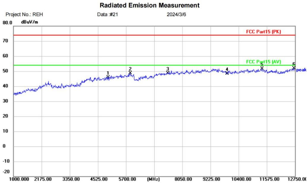
Site Polarization: **Horizontal** Temperature: (C)
