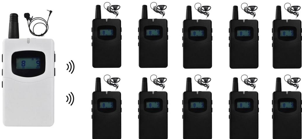
The devices use rechargeable batteries. 70T transmitter can work 25 hours continuously after full charge and 70R receiver can work 60 hours continuously after full charge. Micro USB cables can be used to charge the devices. Be ware of the correct plugging direction. Wrong and violent plugging will damage the charging port in the device. It will take 5 hours for full charge. When the devices are being charged, the light will turn red. When they are fully charged, the light will turn green.
