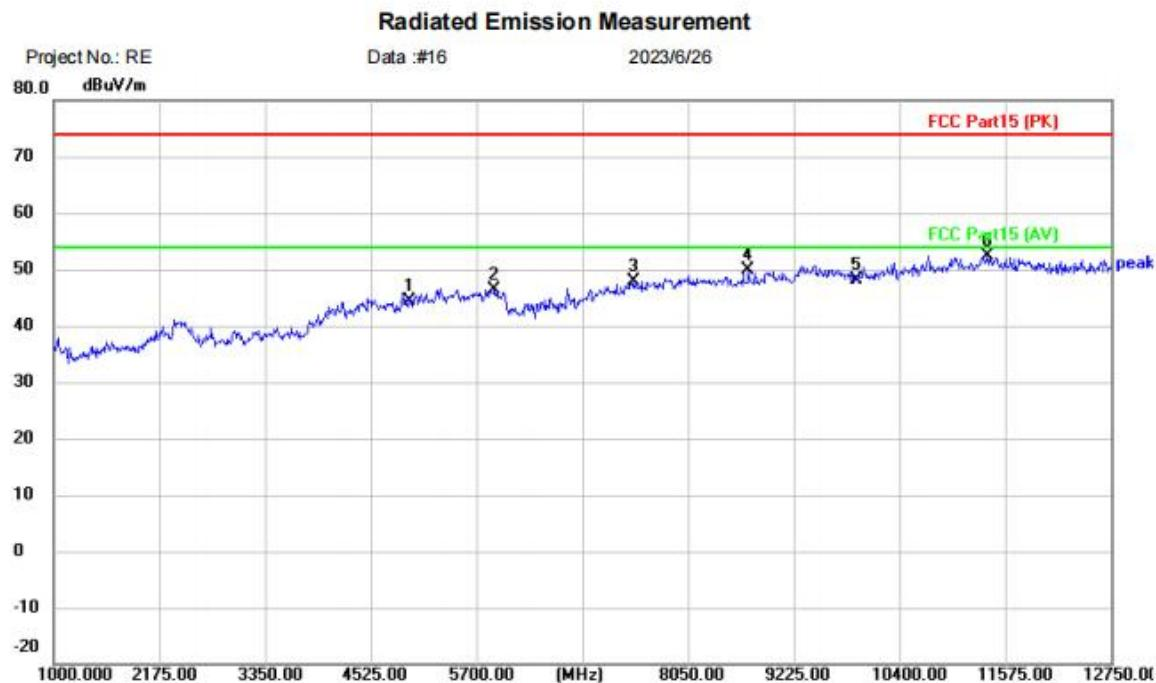
Site: Limit: FCC Part15 (PK) EUT: Sound amplifier M/N: diacovsky CR430S B+ Mode: BLE TX-H Note: Polarization: **Vertical** Power: Temperature: (C) Humidity: %RH
