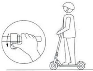
3. Press the accelerator lever slightly, and the scooter accelerate. Put both feet on the board after you can keep balance. Press down the lever to speed the scooter up.
