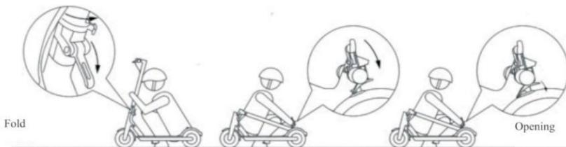
Make sure that the power of electric scooter is turned off, open the folding mechanism, put down the pipe, and hook the handlebars onto the rear fender. When opening you need to press the hook at the rear fender, until the handlebars can be released, then unfold the electric scooter.
