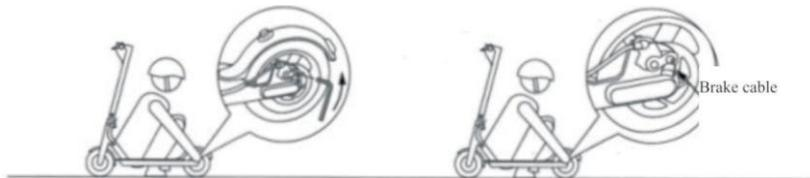
If you feel the brake is too tight, please use the M5 Allen wrench anticlockwise to release the screw on the disc brake, adjust the brake cable to make the tail slightly shorter, and tighten the screw. If you feel the brake is too loose, release the screw, adjust the brake cable to make the tail slightly longer, and then tighten the screw.
