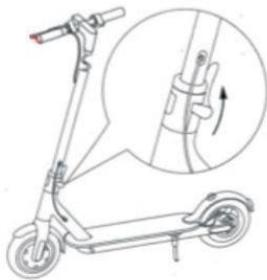
2. Install the handlebars with the pipe.
