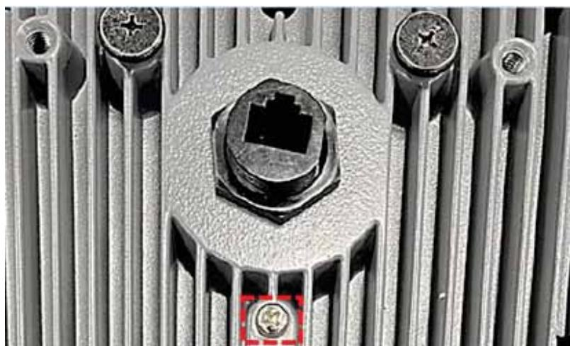
The screw is for earth terminal, it shall be used 18 AWG minimum size with green-yellow conductor to connect to earth.
