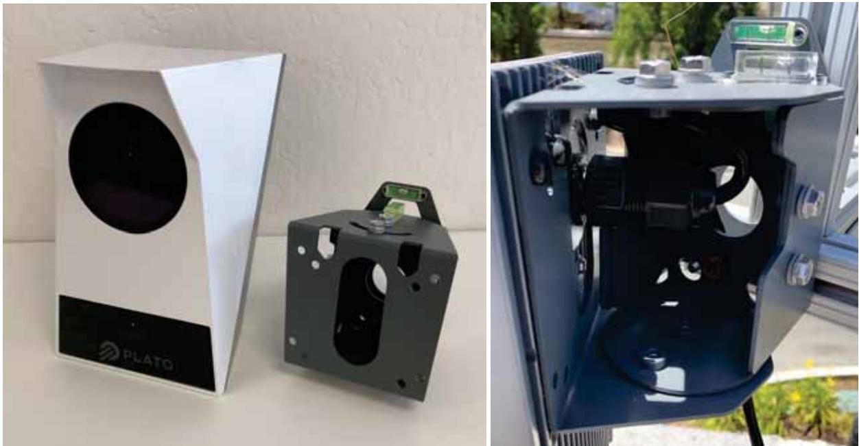
Four screws are used to attach the mount to the mounting surface.
