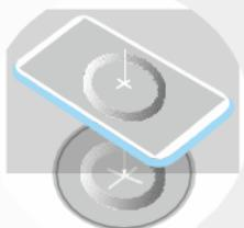
**Put the phone in the center of the charging surface (this lets the charging coil in your phone line up with the one inside the wireless charger).**
