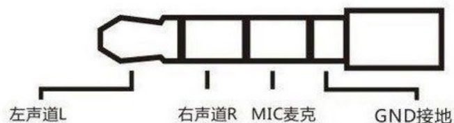
Figure 9Schematic diagram of ido-evb3020 earphone
