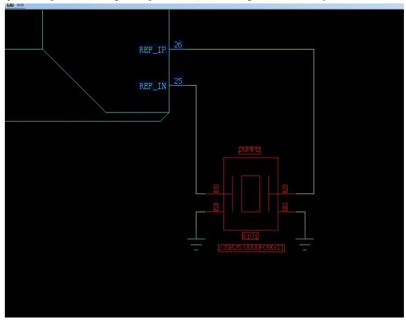
26 MHz is the reference frequency. It is turned on when the supply voltage VTCXO is applied. After buffering a reference clock of 26 MHz is supplied to the other parts of the system through the pin XBUF.
