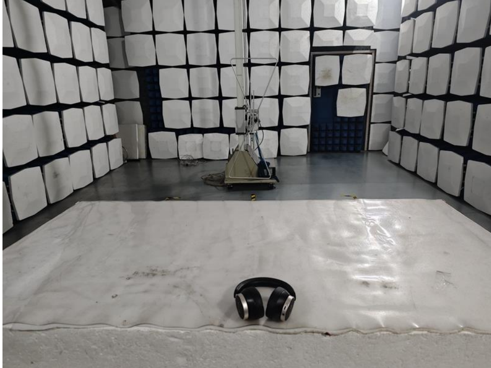
Radiated Emission Test Setup:
