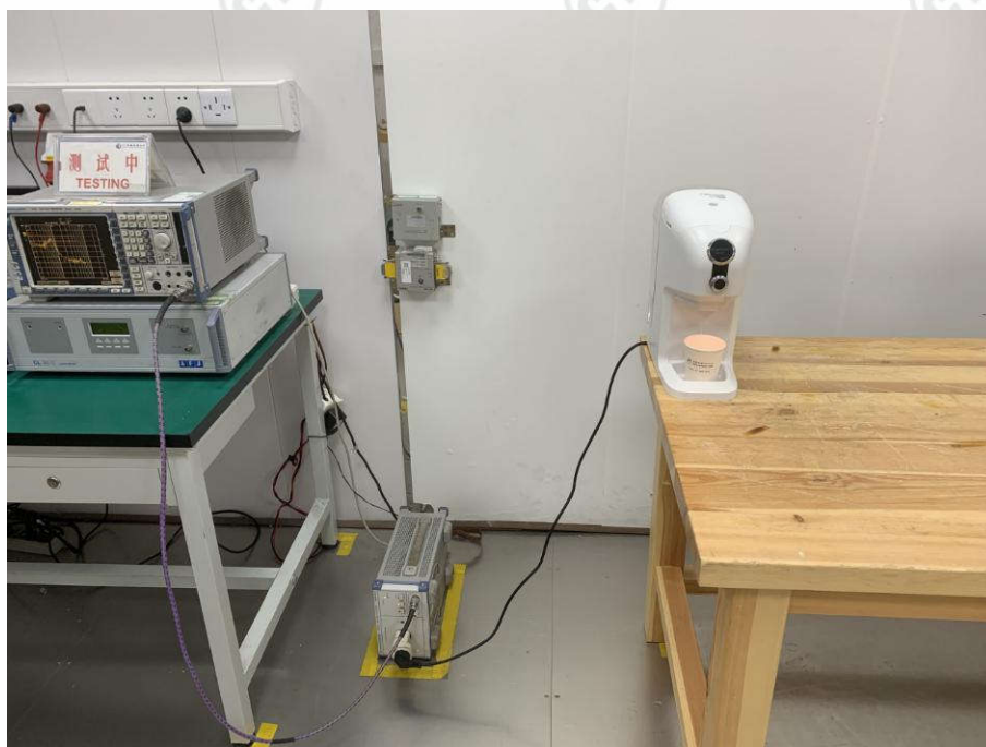
CONDUCTED EMISSION TEST SETUP
