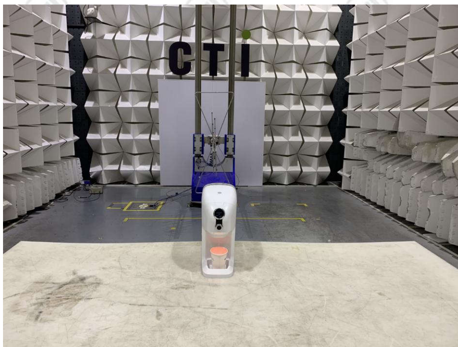
Radiated spurious emission Test Setup-1(Below 1GHz)
