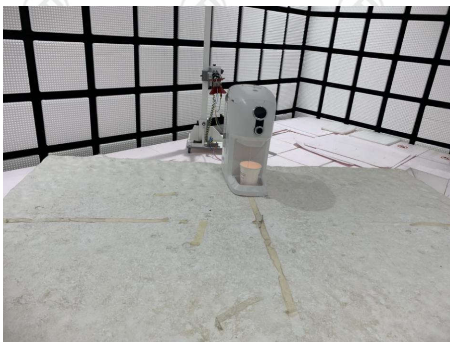
Radiated spurious emission Test Setup-2(Above 1GHz)
