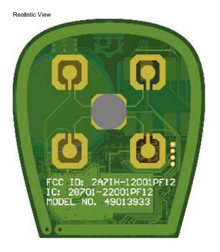
EUT clam shell is removable, so label is silkscreened onto PCB. Visible when battery is installed by end user.
