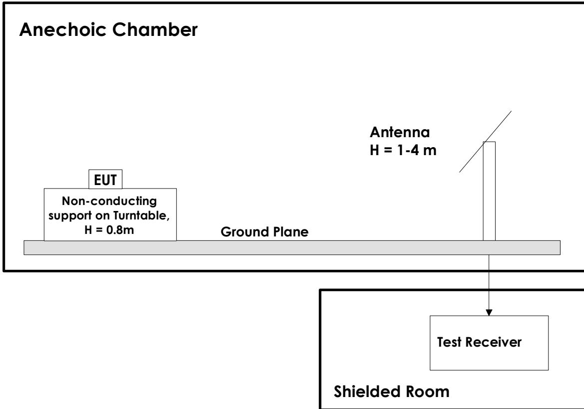
For measurements above 1 GHz the ground plane is covered by absorbers.
