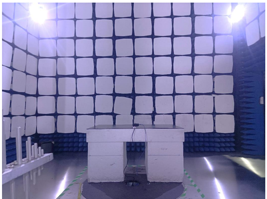
Radiation Emission Test Setup (30MHz to 1GHz)
