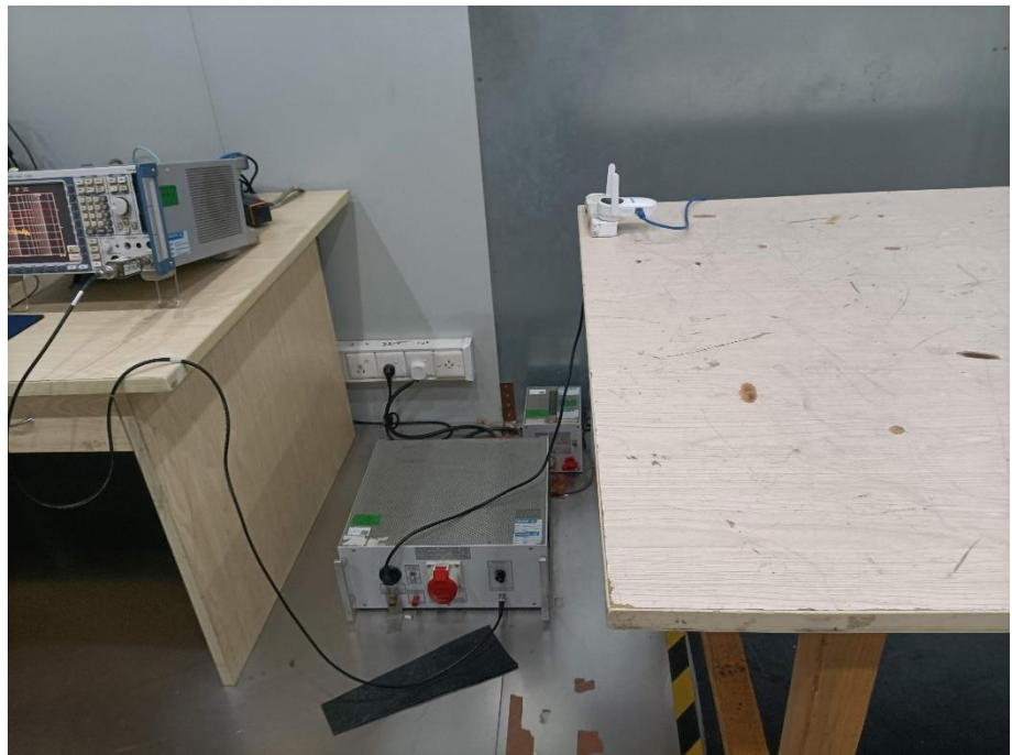
Conducted Emission Test Setup
